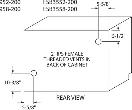
Flammable storage cabinets can be painted any standard color or safety yellow. For synchronized self-closing doors, add -SCC to the part number. For 22" deep, replace -200 with -220. For mobile cabinet, contact your AMS representative.
