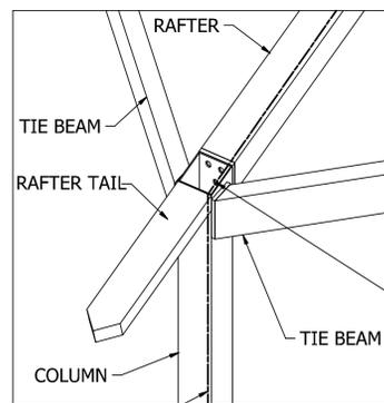
ICON PROVIDES A MINIMUM OF (1) 3/4" HOLE AT EACH CONNECTION FOR 1/2" CONDUIT. IF APPLICABLE, PLEASE SPECIFY REQUIRED CONDUIT SIZE: (CHARGES APPLY)
