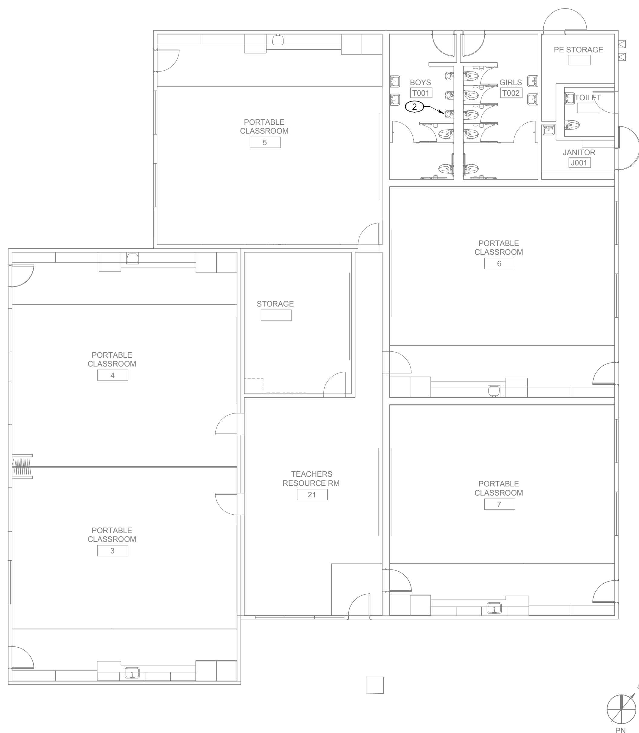
PLUMBING IMPROVEMENT FLOOR PLAN - BLDG 5 2 1/8" = 1'-0"
