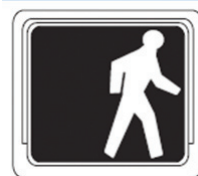
Figure 4. Indicates that the pedestrian may "WALK" or start to cross by entering the roadway.
