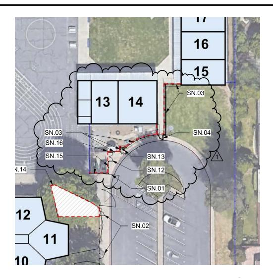
SN.12 (E) PR. GATES TO REMAIN. REMOVE CHAIN LINK FABRIC AND SLATS. PAINT THE (E) GATE FRAME BLACK. INSTALL (N) BLACK VINYL COATED CHAIN LINK FABRIC W/BLACK PRIVACY SLATS
