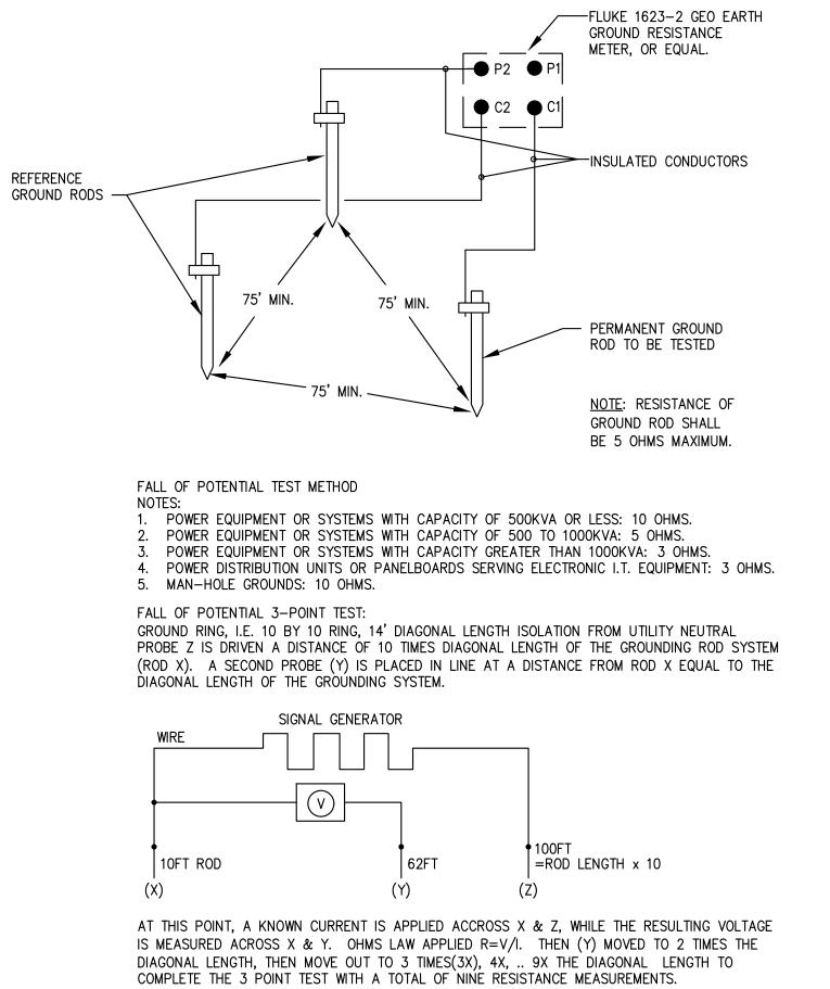
6 METHOD OF TESTING GROUND RODS DETAIL SCALE: NONE
